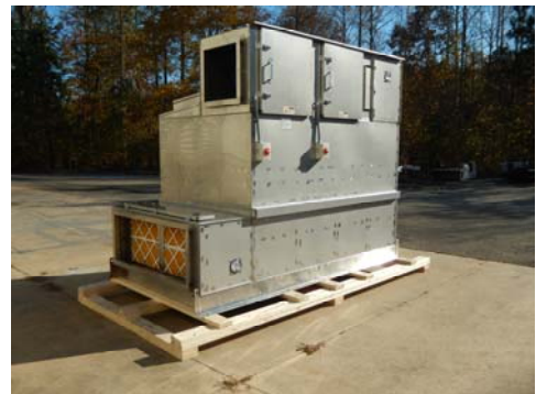
Horizontal bulk fill system with fans in series for simple two stage flow and redundancy. All motors are under cover.
