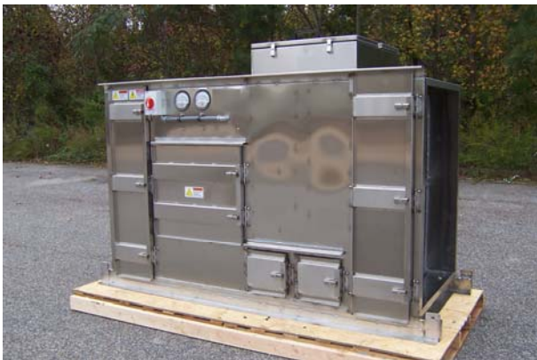
Deep bed scrubber.
