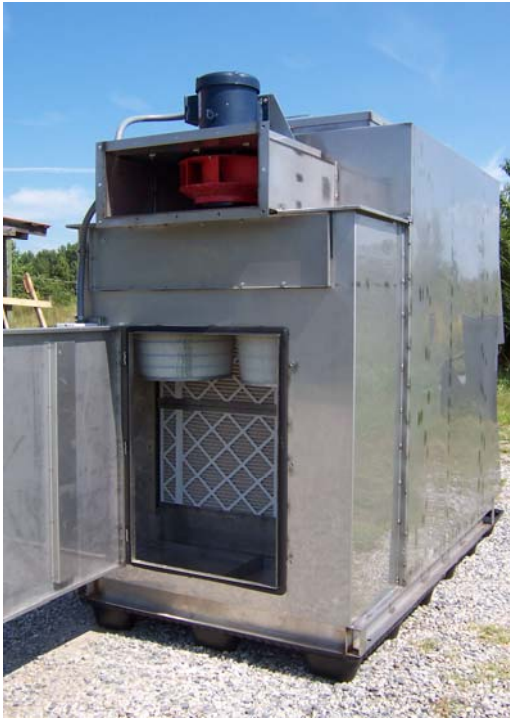
Vertical bed scrubber with cartridge final filters for zero bypass for refinery.
