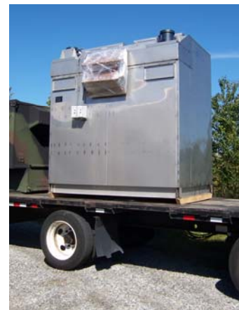
Large vertical bed scrubber with twin fans for ammonia removal at a composting facility.
