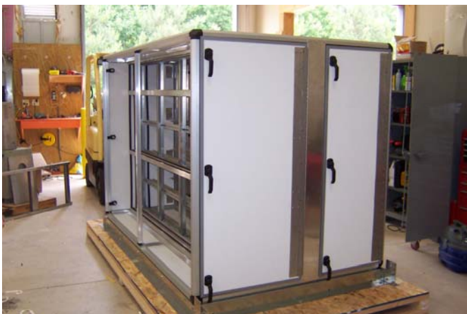
Side access housing. Double wall insulated panels.
