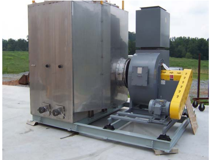
Vertical bed scrubber for wastewater treatment plant.
