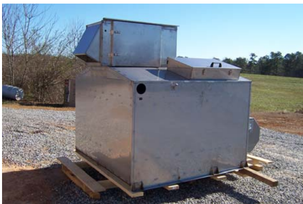
Horizontal bulk fill system with enclosed fan.
